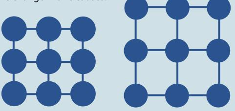
Left: object at low temperature. Right: object at higher temperature. Individual molecules have moved away from each other and the overall volume has expanded.
