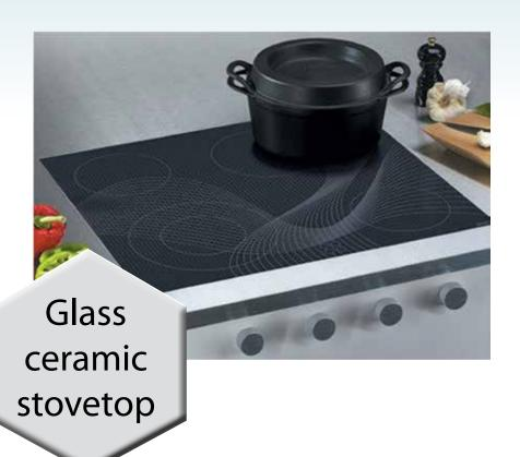
This material is used for stovetops and some cookware because it can undergo heating and cooling cycles without breaking because it has a low coefficient of thermal expansion (CTE). This means it's very reliable, which is important since kitchen items get a lot of use.
