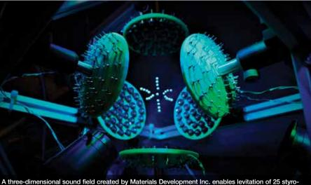
foam spheres. The process allows for measurements using neutron methods to study how liquids change into glass and to investigate extreme temperature processes. Credit: Materials Development Inc.
