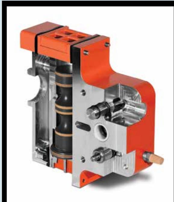
The Wilden Pro-Flo SHIFT Air Distribution System revolutionizes AODD pump operation through a design that reduces air consumption by up to 60% when compared to competitive models. *Credit: Wilden*
