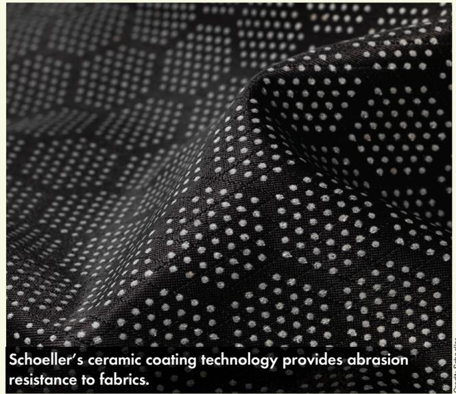
Schoeller's ceramic coating technology provides abrasion resistance to fabrics.
