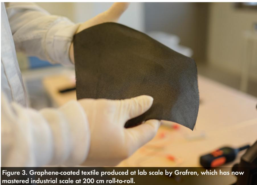
Figure 3. Graphene-coated textile produced at lab scale by Grafren, which has now mastered industrial scale at 200 cm roll-to-roll.
